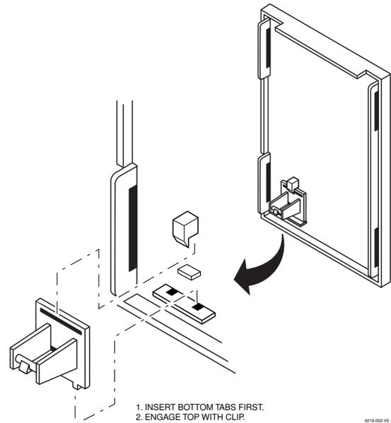
**Figure 1. Tamper Magnet Installation**
